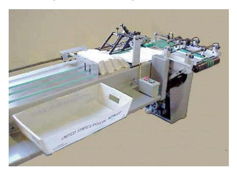
Automatic sorting combined with edge stacking makes mail tray filling quicker and easier.
